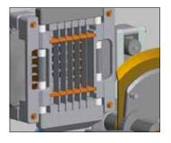
The intelligent vartronic technology is important, especially when frozen meat is diced. The machine is able to adapt its cutting tools if products are too cold or too hard – thanks to separate drive mechanisms for the lower grid, upper grid and blade.
