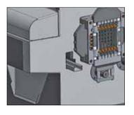
TWISAN is equipped with multiple collection devices and gutters. They allow, for example, drainage of meat juice away from the meat or feed it back to the final product. This also shows the sophisticated hygienic design again.
