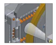
Sensors control the frequency of the blade in order to achieve exactly the desired cube or strip size. The result is a convincingly clear cutting pattern and a high output. The sensor as well as a number of operating modes (for example, the dual lateral compression) can be switched on and off as required.
