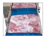
The machine can cut blocks of frozen meat into cubes or strips of up to 50 mm /2" in length.
