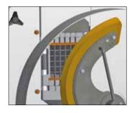
The cutting area is equipped with a new scraper. This not only prevents the bulk material from being contaminated with product residues. Even the cutting area also remains much cleaner.
